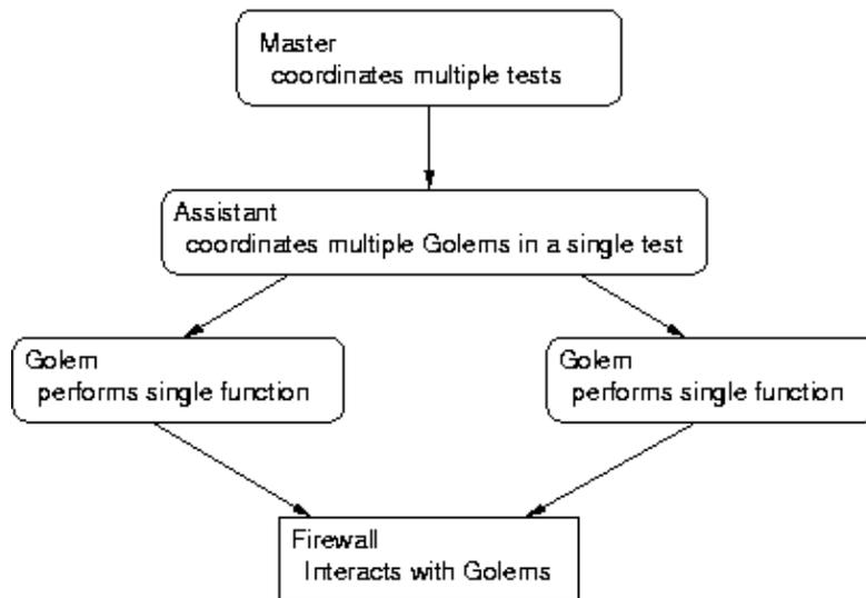
The Master process spawns an Assistant for each test. The Assistant coordinates one or more Golems which perform single functions like probing or monitoring the system under test.
