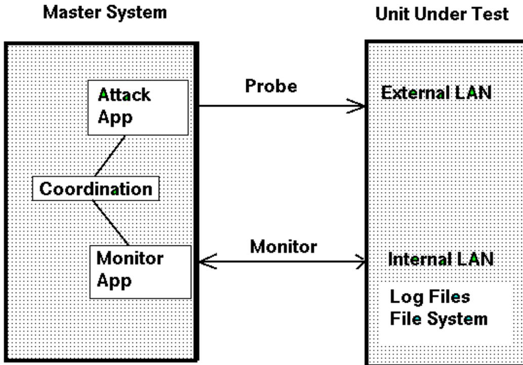
Coordinated probing and monitoring of the system under test provides complete assessment of the systems behavior
